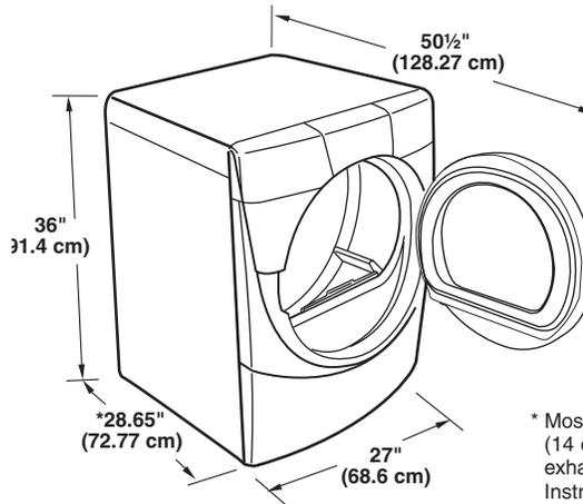
\* Most installations require a minimum 5/2" (14 cm) clearance behind the dryer for the exhaust vent with elbow. See Installations Instructions, "Venting Requirements."
