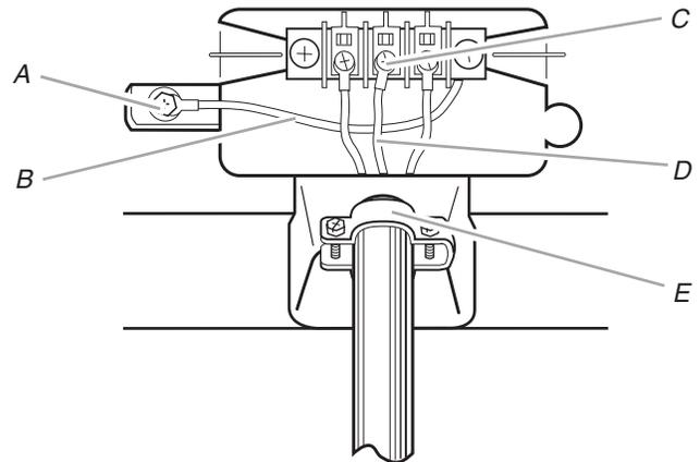
A. External ground conductor screw
