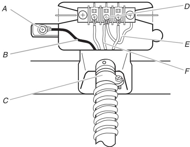
A. External ground conductor screw
