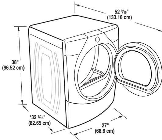
\*Most installations require a minimum 5" (12.7 cm) clearance behind the dryer for the exhaust vent with elbow. See "Venting Requirements."
