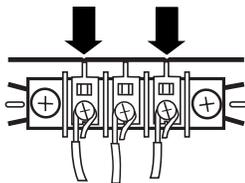
4. Tighten strain relief screw.
