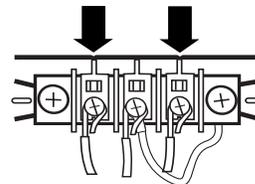
4. Tighten strain relief screws.
