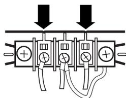
5. Tighten strain relief screws.
