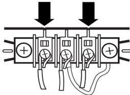
5. Tighten strain relief screw.
