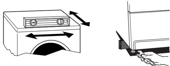
If the dryer is not level, prop up the dryer using a wood block. Use a wrench to adjust the legs up or down and check again for levelness.
