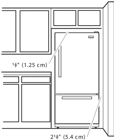
To ensure proper ventilation for your refrigerator, allow for 1/2" (1.25 cm) space at the top and behind the refrigerator for ease of installation.
