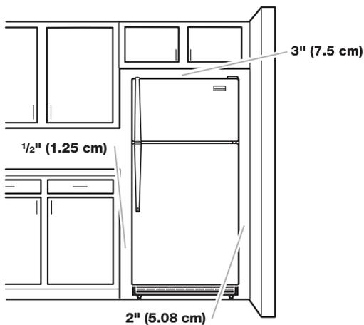
To ensure proper ventilation for your refrigerator, allow for 1/2" (1.25 cm) space on each side. Allow 3" (7.5 cm) of space between overhead cabinets and refrigerator top. When installing your refrigerator next to a fixed wall, leave 2" (5.08 cm) minimum on the hinge side (depending on your model) to allow for the door to swing open. If your refrigerator has an ice maker, allow extra space at the back for the water line connections.
